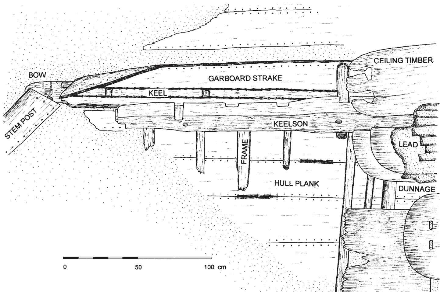
Fig. 78 Detail of the hull remains near the bow.
